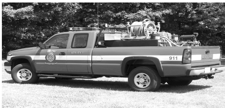
Rye Fire Department's newest piece of apparatus: Chevrolet 4x4 pickup with 225 gallon water tank, fire pump, and hose reel.
