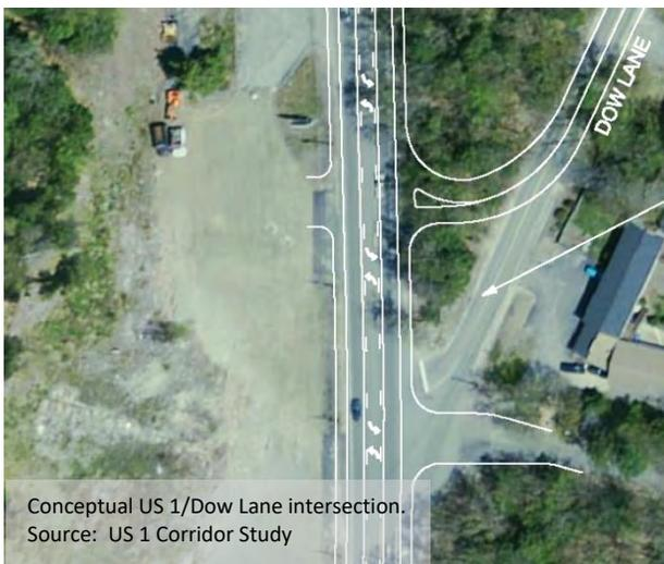
Figure 12: US 1/ Dow Lane intersection. Top Left - Existing layout, Bottom Left - US 1 Corridor Study concept, Right – Current conceptual layout working within existing right-of-way.
