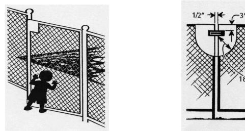
Gate must *swing out* and be *self-closing & self-latching*. When the release mechanism is less than 54" from bottom of gate, it must be at least 3" below the top of the gate and located on the side of the gate facing the pool. There must be no opening in the gate greater than  $\frac{1}{2}$ " within 18" of the release mechanism.
