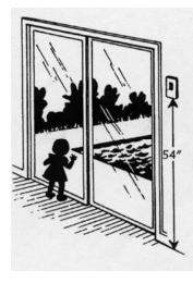
Doors with direct access to the pool must be equipped with alarms meeting Appendix G requirements (alarms meeting UL 2017 are acceptable). Door alarms associated with home security systems will not usually meet these requirements. This does "**NOT**" replace the requirement for Pool Barriers.
