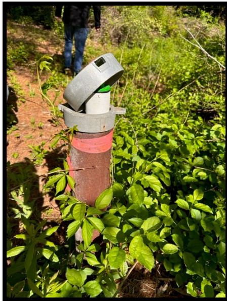
Photo 2: PVC riser sticking out of casing MW-101
