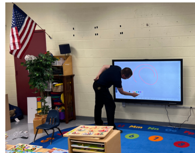
An interactive panel installed in a pre-school classroom. Note they are installed much lower for Pre-K and K so students can reach them.
